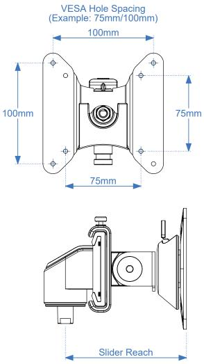
Measure distance from the stem pivot point's centerline up to the VESA plate.
