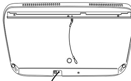
After wall-side bracket is mounted, have a second person help lift the air purifier and prepare to mount it to the wall bracket. Lift the machine up so the machine-side bracket is above the wall-side bracket. Tilt the machine to about 45 degrees and lower it until the machine-side bracket rests on the wall-side bracket.
