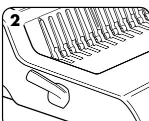
2. Insert the plastic comb into the mechanism.
