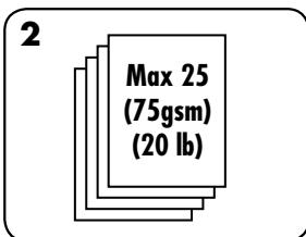
2. Punch sheets in small batches that do not overload the machine or the user. Adjust edge guide, if necessary.
