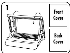
1. Ensure edge guide is set to the proper document size. Punch front and back covers first.
