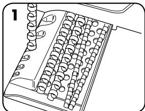
1. Select the correct comb diameter using the comb storage tray.
